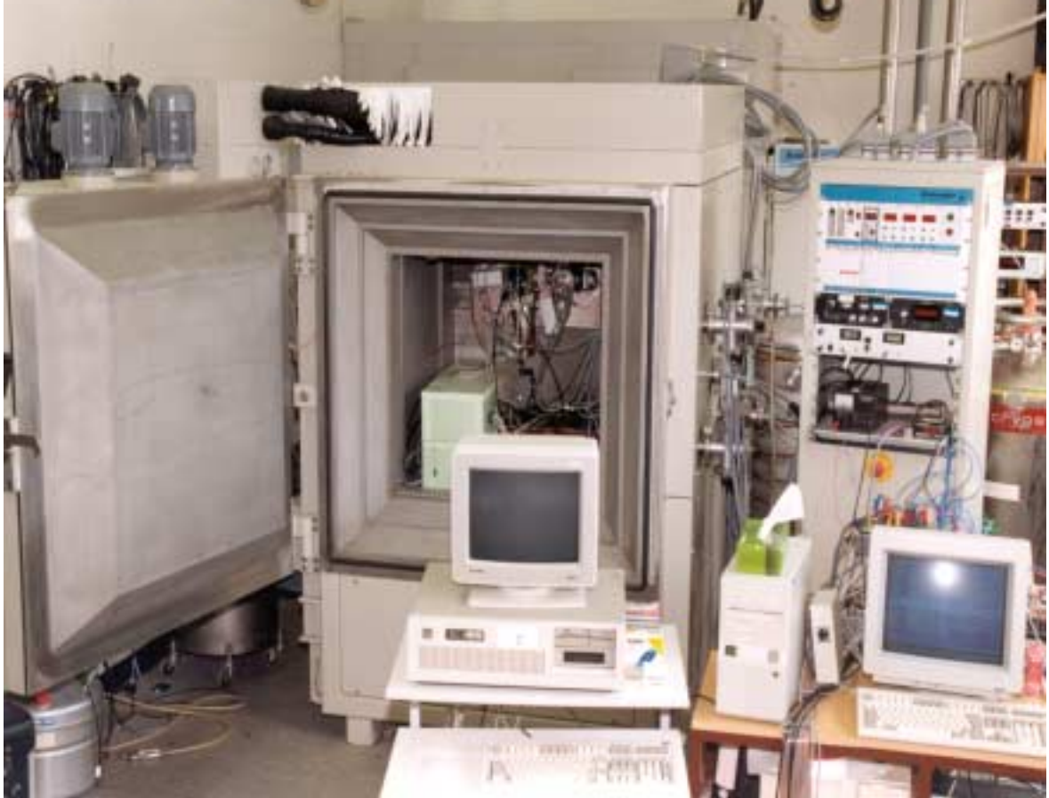
Figure 1: Environmental Simulation Chamber (ESC) at Research Centre Jülich (ICG-2)
