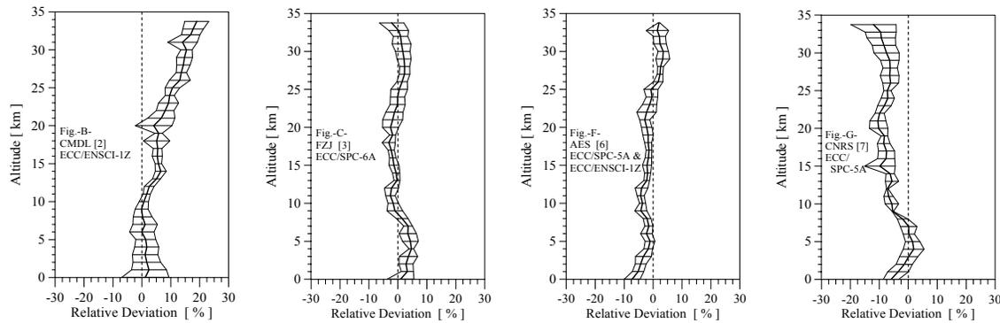
**Figure 1: JOSIE-1996 comparison of ECC-sondes. Average (thick line) plus/minus one standard deviation (thin line) of the relative deviations of the individual sonde readings from the UV-photometer for each participating ECC-sounding laboratory obtained from six simulation runs. For details see Smit and Kley [1998].**
