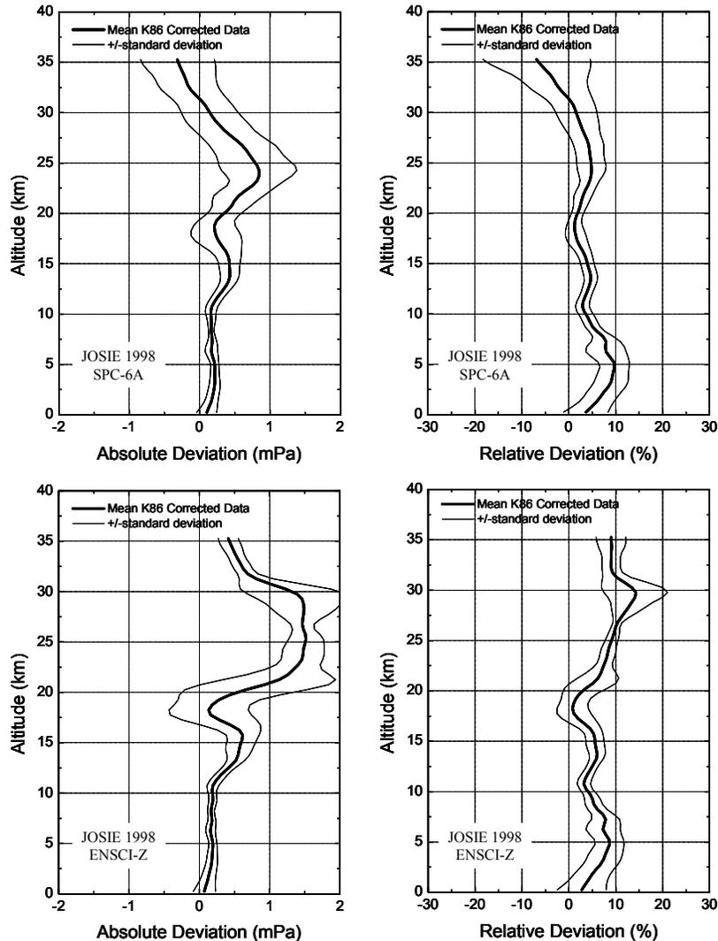
**Figure 3: JOSIE-1998 comparison of all (13) tested SPC-6A (upper diagrams) and all (13) tested ENSCI-Z ozone sondes (lower diagrams). Results presented as averages ( $\pm$  one standard deviation) of the ozone pressure deviations (left diagrams) and as averages ( $\pm$  one standard deviation) of relative deviations (lower left and right diagram) of the individual sonde readings from the UV-photometer, respectively.**
