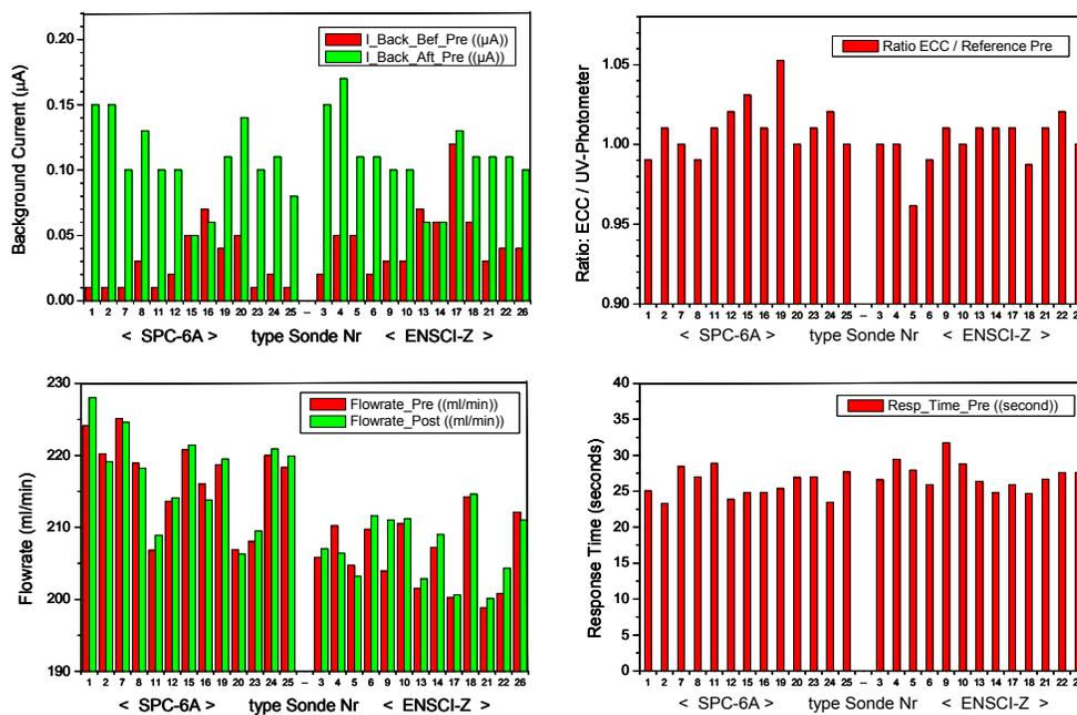
**Figure 2: Results from pre-flight tests of the performance of the “flown” ECC-sondes. Left upper diagram: Background current of ECC-sensor before and after exposure with ozone. Right upper diagram: Conversion efficiency of ECC-sensor compared to UV-photometer. Left lower diagram: Flow rate of gas sampling pump at pre-and post- flight simulation. Right lower diagram: Response time of ECC-sensor. For details see text.**
