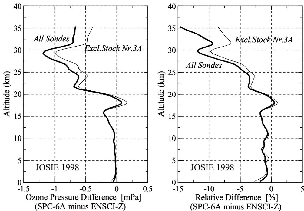
**Figure 5: JOSIE-1998 comparison of the absolute (left diagram) and relative (right diagram) differences between SPC-6A and ENSCI-Z sondes derived from the differences of the average deviations of the SPC-6A and ENSCI-Z sondes with the UV-Photometer as presented in the Figures 4 and 5 for all tested SPC-6A sondes (fat line) and excluding the sondes of stock nr. 3A (thin line), respectively.**
