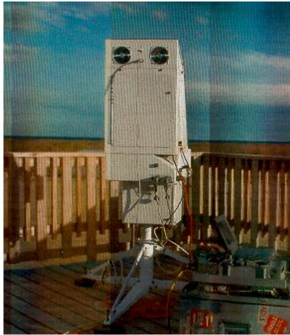
Figure 4.1.2 The Brewer “dog house” for in situ calibrations.
