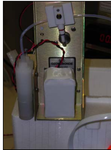
Figure 19 - Battery attached to ozonesonde with cables underneath the cathode tube
