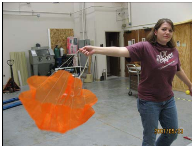
Figure 13 - Fluff out parachute by swiftly pulling it behind you
