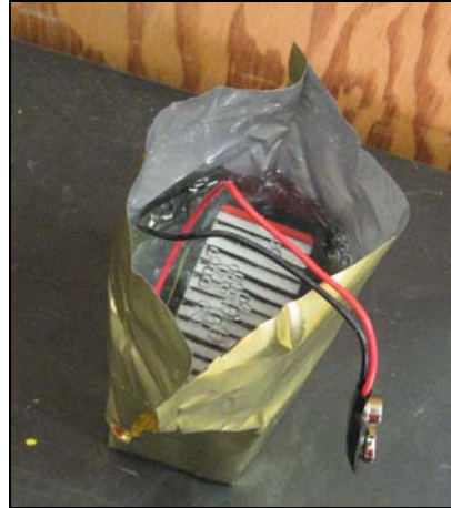
Figure 23 - Wet battery bag with water filled above the battery
