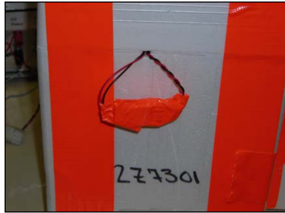
Figure 26 -Once connected wrap cables with tape
