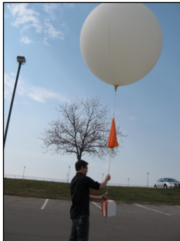
Figure 31 - Release the balloon and parachute first; make sure the strings are not tangled
