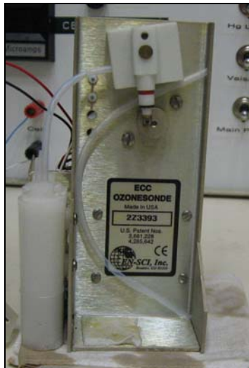
Figure 1 - The feeder tube is slid into the space between the motor, making a “C” shape
