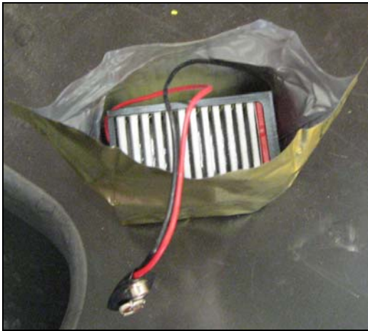
Figure 22 - Wet battery with cables out of bag
