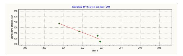
After the above sun scan tests the cal step was adjusted to step 292 on #110. The graphs below show a normal slit function and that the UV sensitivity has decreased by 10% since 2001.
