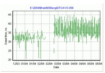
Below are SL, DT and other graphs of **Brewer #124**, normally located at C. Paulista site. Note the somewhat unstable SL ratio R6 and stable DT results since 2002. Note the decrease in sensitivity of 20-24% since 2000, which is shown in internal standard lamp and external UV lamp scan test results.. The sun scan results show cal step 290 is proper.
