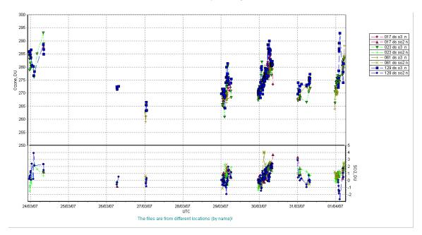
Below are the ozone and Aerosol Optical Depth (AOD) results from the same direct sun measurements for the last 4 days. Each instrument was using the following AOD ETC constants, (etc06.023, etc06.061 and etc04.129). The revised control software (V376A) calculates AOD in real time with the use of new AODVAL.nnn files for each instrument.
