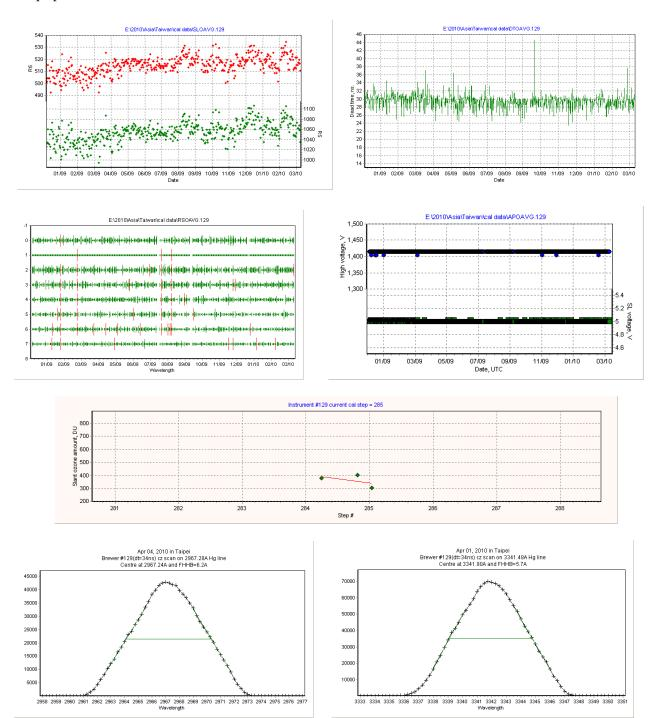
Below is a graph of the UV response file UVR09210.129 and in second graph it is compared to the in use file UVR08808.129, which was not changed due to the small differences.
