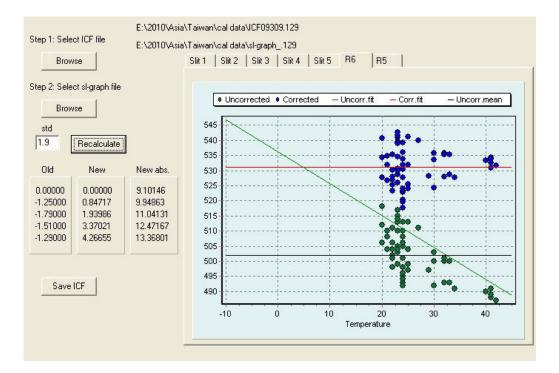
Original temperature range: 20 - 42 from the period: Mar 31 2010 to Apr 05 2010 Mean SL ratios R6/R5 before correction = 502 / 1019; after correction = 531 / 1091Final constants for slits 1-5 are: 9.1015, 9.9486, 11.041, 12.472, 13.368
