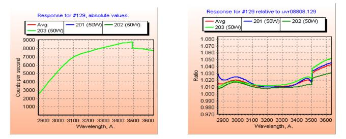
New temperature coefficients were calculated for #129 as shown below and are included in file (icf09510.129), which was put into use during this visit. The new SL ratios are 530/1090 and final ETC constants are 1800/815. Reference final graph from TCPRO program which shows temperature dependence (green dots) and recalculated R6 ratio results (blue dots).
