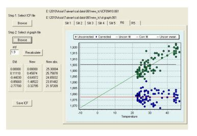
> Opposite is graph from TCPRO program which calculated new temperature coefficients for #061 using SL results from the period: Apr 03-12, 2010 temperature range: 22 - 47
