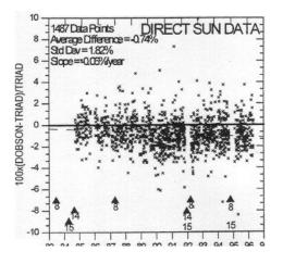
Figure 2.1.3 The ratio of Dobson instrument #77 AD direct sun daily ozone values to the daily triad values over the twelve-year period. The average ratio is 0.9926 with a standard deviation of 0.0182. The slope of the best fit (dashed) line is -0.0006 per year (-0.6% per decade).
