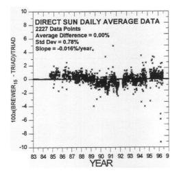
Figure 2.1.2 The ratio between ozone measured by Brewer instrument #15 to the triad ozone value. The average ratio is 1.0000 with a standard deviation of 0.0078. The slope of instrument #15 compared with the triad (dashed line) is -0.00016 per year (-0.16% per decade).
