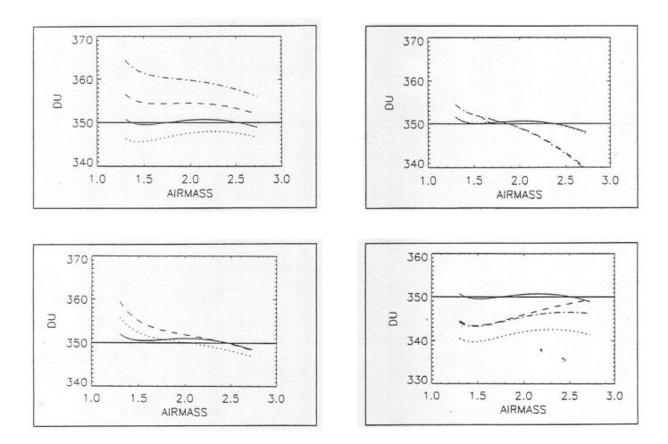
Figure 2.3.2 Results of the sensitivity study of the global ozone measurement method. The first figure shows the effect of albedo, the second the effect of aerosols, the third shows the effect of various cloud optical thickness and the fourth shows the effect of various ozone profiles.
